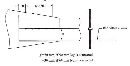
Determine the tensile strength of a roof truss member 2 ISA 90mm x 60mm x 6mm connected to the gusset plate of 8mm plate by 4mm weld as shown in fig. The effective length of weld is 200mm.
