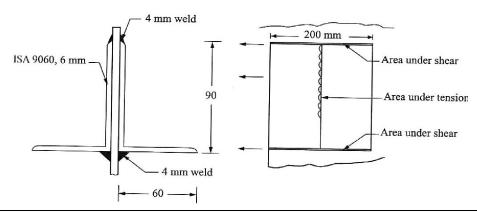
Design a single angle section for a tension member of a roof truss to carry a factored tensile force of 205 KN. The member is subjected to the possible reversal of stress due to
