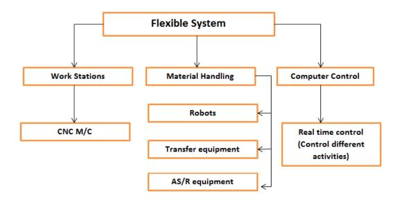
Processing work stations- The work stations that perform different operations on part families are called processing stations. These work stations are CNC machine tools, inspection equipments, assembly system, inspection system, lead changers and loading/unloading area.
