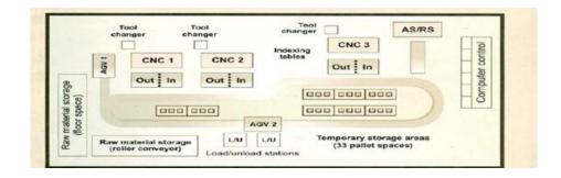
Material handling system – It is used to move the material or parts from one machine to another machine and from machine to storage point etc. These systems include automated guided vehicles, roller conveyor, robots etc.
