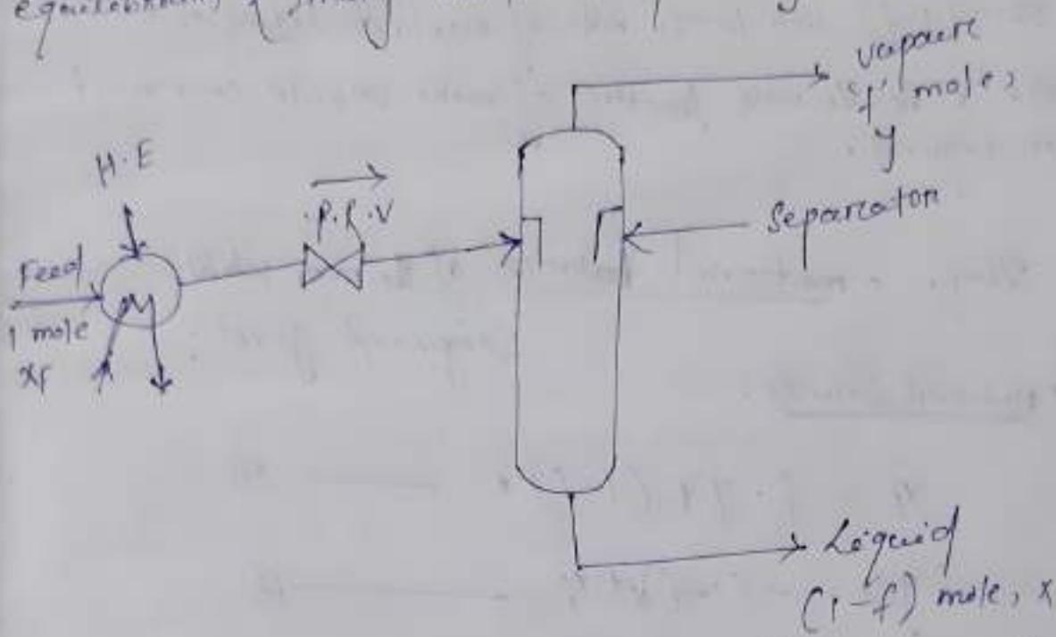
Feed is heated in a tubular heat exchanger. The hot liquid mix. is then fed to a separator via pressure reducing valve whereby pressure is reduced & the vapour is formed at the expense of liquid adiabatically. The liquid is withdrawn from the bottom of the separator & the excess vapour leaves the separator from the top which is then liquefied in a condenser. Flash distillation is commonly used in petroleum industry, handling multi component systems in the pipe mills.
